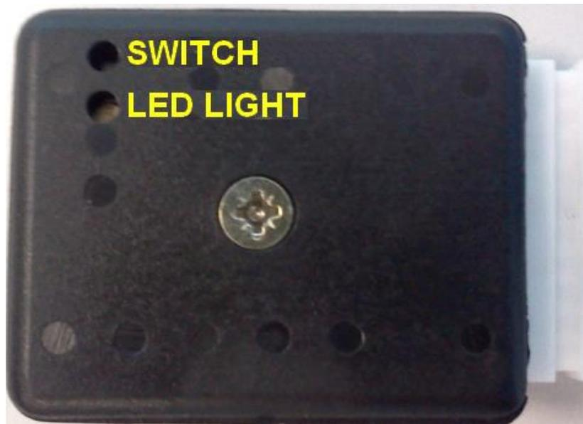
Figure 52 Adapter signaling led
